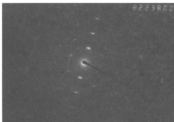
Fig. 10 SAED of \text{CeO}_2 -5 wt. % \text{Yb}_2\text{O}_3 irradiated for 7 s and energy density of 17.18 \text{ kJ}\cdot\text{cm}^{-2}
